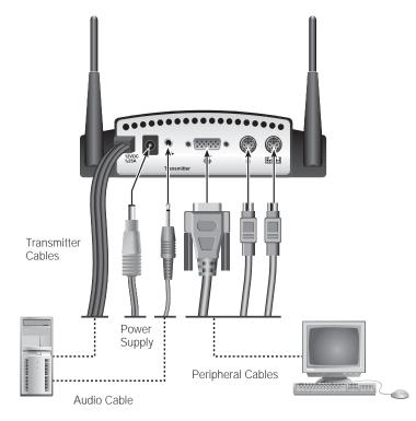
Figure 2.1: LongView Wireless Transmitter Installation Example
